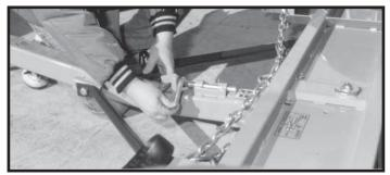
**Step 3.** To allow the wheel platform to tilt back for loading: 1) Swing the bottom of the locking latch (C) toward the hitch far enough to allow locking pin handle to be lifted.
